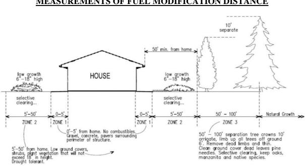
**<u>FIGURE 4907.2</u>** MEASUREMENTS OF FUEL MODIFICATION DISTANCE
